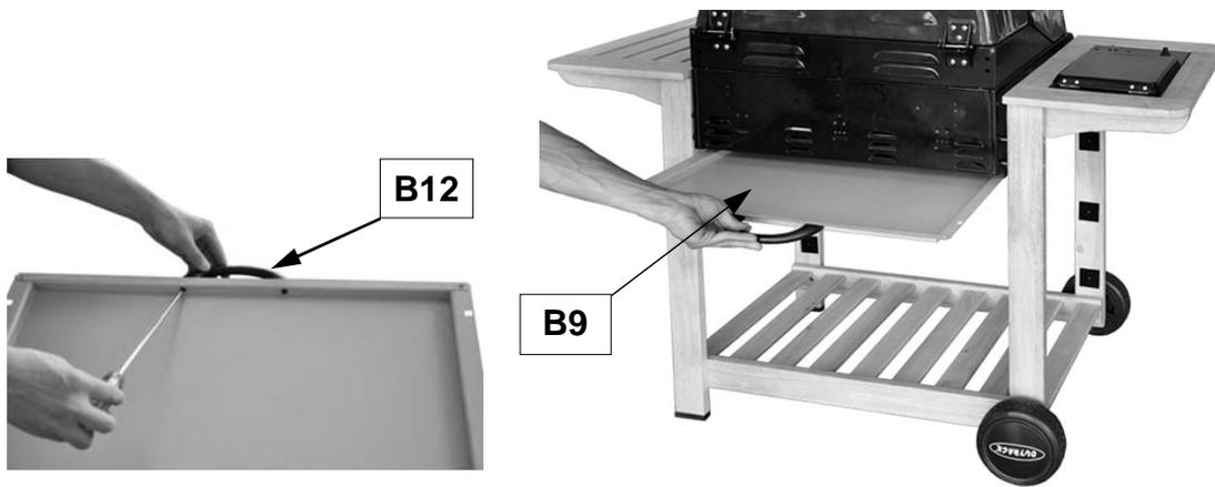
Remove the retaining screws from Drip Tray Handle (B12), then attach the drip tray handle onto Drip Tray (B9) with the retaining screws. Insert the drip tray by sliding it underneath the barbecue body.
