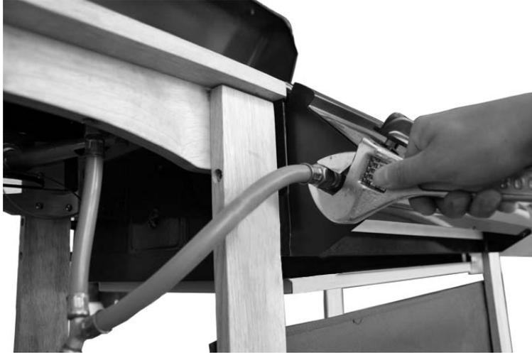
Connect the Hose and Regulator Assembly (B13) to the side burner gas inlet and main burner gas inlet. Ensure the mating faces of the connections are clean and not damaged. Do not use any sealing tape, paste or liquid on the joint. The nut must be tightened with a spanner. Do not use force which may damage the assembly.
