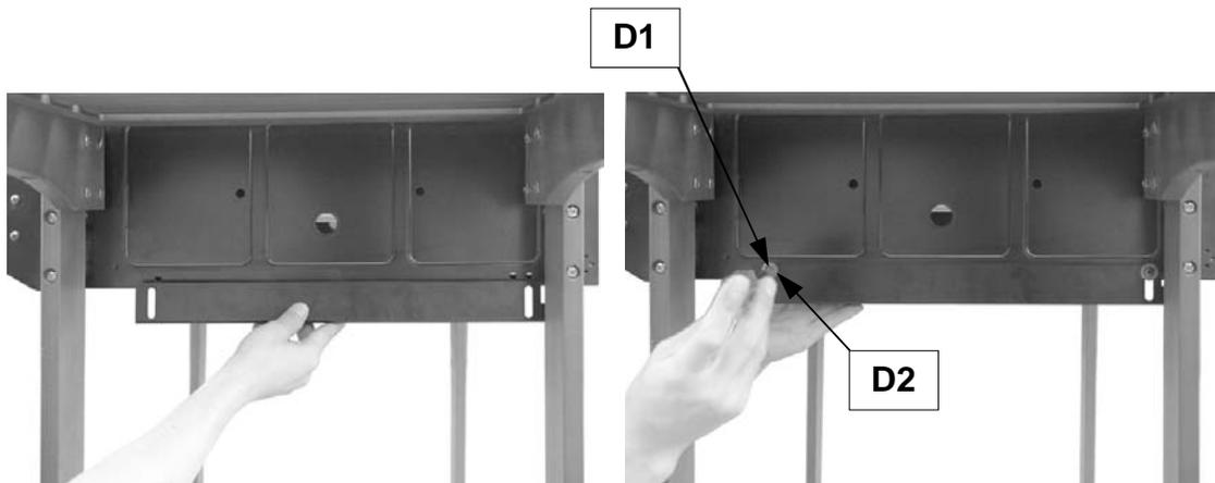
Attach Drip Tray Right Bracket (B11) to barbecue body using M5x15 Bolts (D1), Ø5 Washers (D2) and M5 Nuts (D3) as shown. Repeat above process for Drip Tray Left Bracket (B10).
