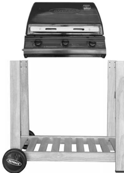
Carefully stand the barbecue upright. Insert M6x95 Bolts (D5) through the trolley legs, the Spacers (D6), and keep the tip of the bolts inside the spacers. While holding the barbecue body into position (2 people required), screw the bolts into the barbecue body as shown.
