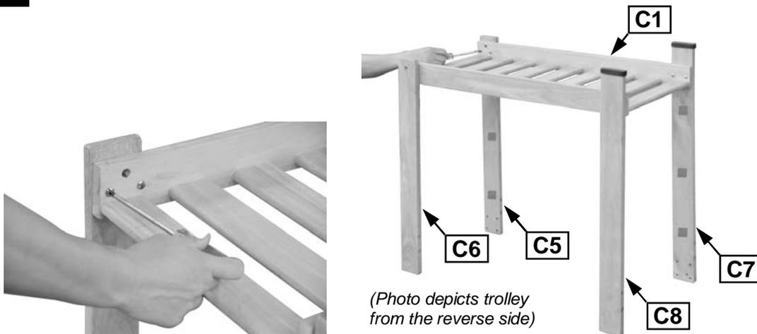
Attach the Legs (C5, C6, C7, C8) to the Trolley Base (C10) using 1/4-20UNCx22 bolts (D4). Ensure that the legs with the Velcro attached to them are at the front of the barbecue, facing inwards.
