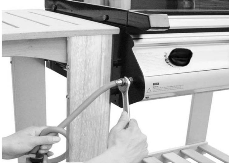
Connect the hose and regulator (B13) to the BBQ. Ensure the mating faces of the connection are clean and not damaged. Do not use any sealing tape, paste or liquid on the joint. The nut must be tightened with a spanner. Do not use force which may damage the assembly.
