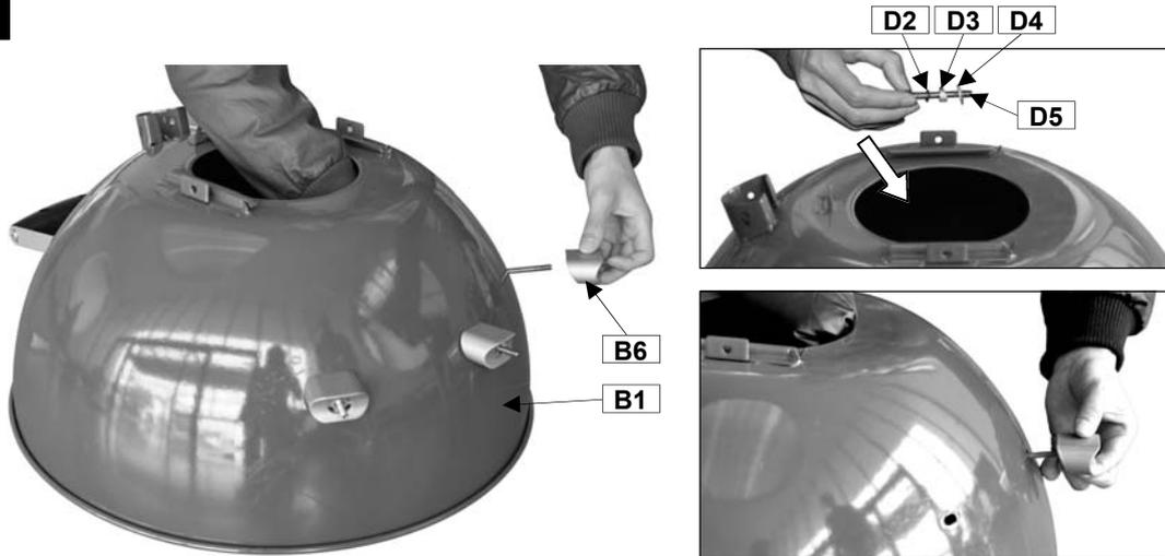
Attach the Heatproof Spacer (B6) onto the Barbecue Body (B1) by inserting M6x50 Bolts (D5x3pcs) through Spring Washers (D2x3pcs), Spacers (D3x3pcs) and Ø6 Washers (D4x3pcs), through barbecue body, as shown.
